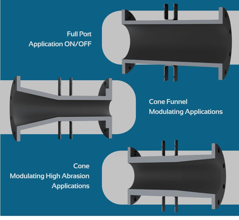
Sleeve sizing program available to determine the proper sleeve for each application.
